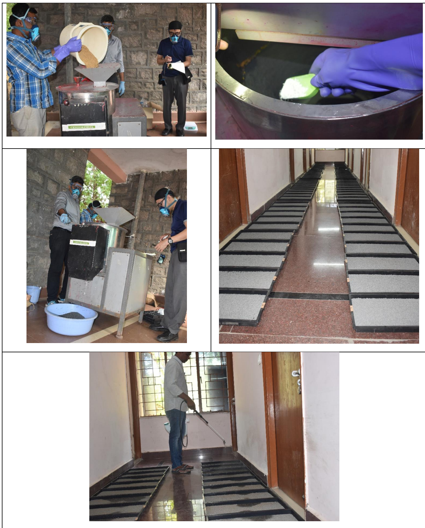
Plate 1: Coating the seed with iron by seed coating machine
